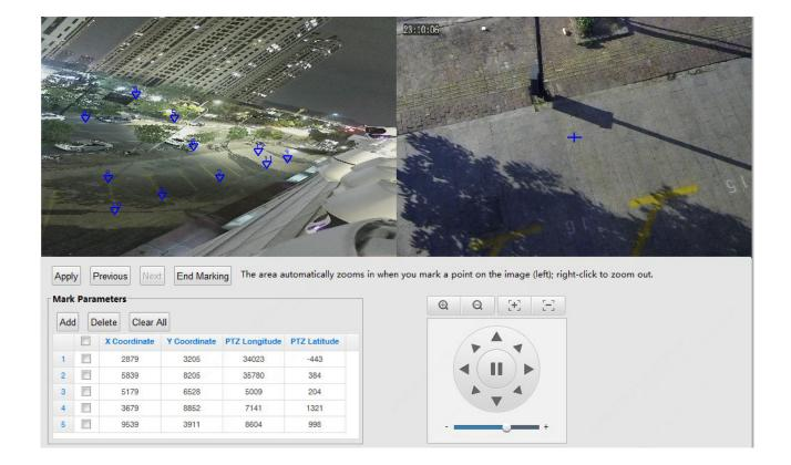
Master-Slave Linkage Use master-slave linkage to link a master device and a slave device. The master device detects the target and the linked slave device tracks and captures the target.
