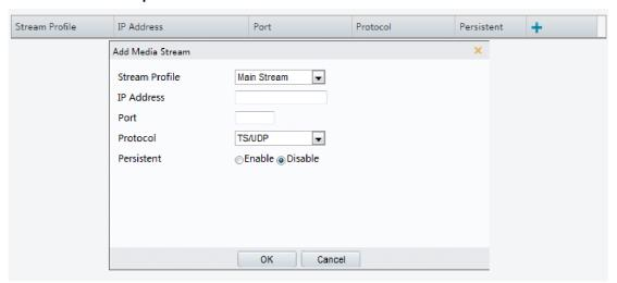
2. Click , select a stream type, and then set the IP address and port number of the unicast or multicast group for the decoding device that receives audio and video streams from the camera.
