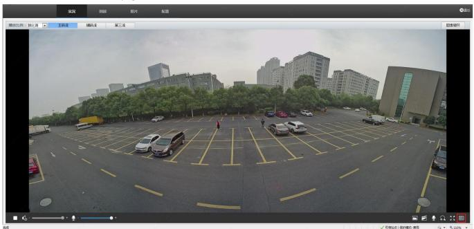
2. When you click in panoramic mode, the live view would change to the 5ePTZ tracking mode. Then camera would detect moving objects in the live view when perimeter protection function is enabled, besides, it can trackand enlarge 5 targets that trigger the alarm rule which you set up in perimeter protection functionat most simultaneously. This function performs like a PTZ camera's tracking and zooming feature.
